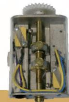
It can be handy adjusted to the required position, setting the chain travelling limits and offering the preventable method for hoist from over winding and damage.
